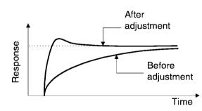
To suppress vibration with a period longer than the value of "H23 I-gain," increase the value of H23.
