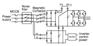
Figure 2-3-2 Connecting the auxiliary control-power input terminals
