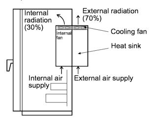
Figure 2-2-2 External cooling system
