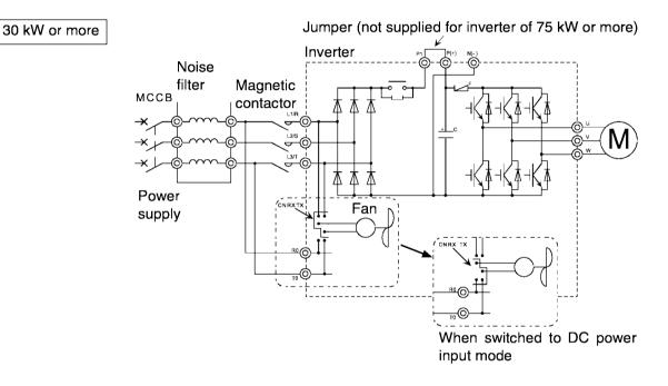
Figure 2-3-6 Fan power switching
