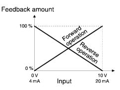
Only positive values can be input for this feedback amount of PID control.
