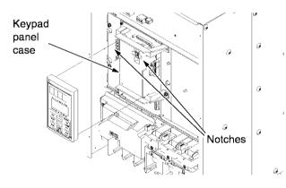
Figure1-3-4 Removing the keypad panel (for inverter of 30 kW or more)
