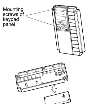
Figure 1-3-3 Removing the keypad panel
