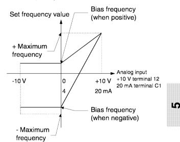
When this function is used with function F17 (bias frequency), the gain set with this function is valid and the gained frequency is biased.
