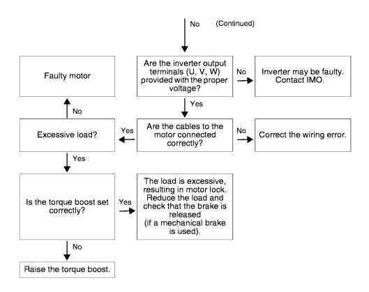
**Note:** Monitor the operation command or frequency setting values, etc., on the LED or LCD monitor after selecting the respective functions. The motor does not rotate if the following commands are issued:
