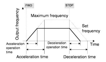
**Note:** If the set acceleration and deceleration times are too short even though the resistance torque and moment of inertia of the load are great, the torque limiting function or stall prevention function becomes activated, thereby prolonging the operation time beyond that stated above.
