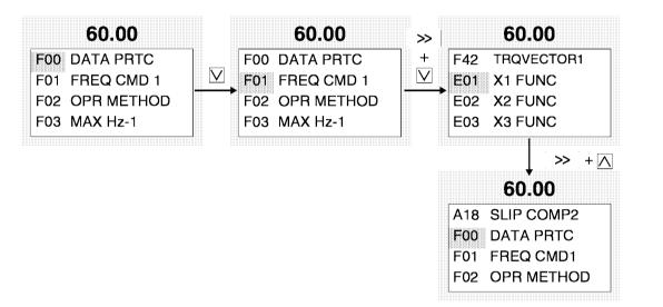
Select the desired function and press  $\frac{\text{FUNC}}{\text{DATA}}$  to switch to the "data setting" screen.
