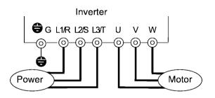
Figure 3-1-1 Inverter connection
