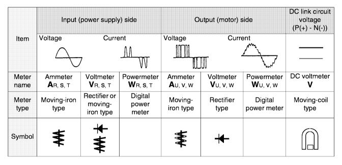
Table 8-3-1 Meters for measuring main circuit
