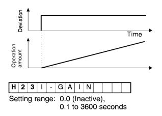
"H23 I-gain" is used as a parameter to determine the effect of I operation. A longer integration time delays response and weakens resistance to external elements. A shorter integration time speeds up response, but an integration time that is too short causes vibration.
