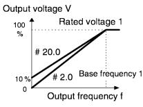
**Note:** As a large torque boost value creates overexcitation in the low-speed range, continued operation may cause the motor to overheating. Check the characteristics of the driven motor.
