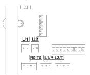
**Note:** To remove a connector, unlock the connector (using the locking mechanism) and pull. To mount a connector, push the connector until it click locks.
