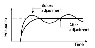
To suppress vibration with a frequency roughly equivalent to the value "H24 D-gain," decrease the value of H24. If there is residual vibration with 0.0, decrease the value of "H22 P-gain."
