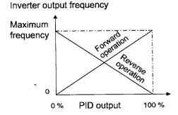
The target value can be entered using F01, "Frequency command 1," or directly from the keypad panel. Select any terminal of Terminals X1 (E01) to X9 (E09) and set value 11 (frequency setting switching).
