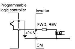
Figure 2-3-11 Connection for External power supply
