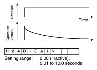
"H24 D-gain" is used as a parameter to determine the effect of a D operation. A longer differentiation time causes vibration by P operation quickly attenuating at the occurrence of deviation. Excessive differentiation time could cause vibration. Shortening the differentiation time reduces attenuation at the occurrence of deviation.
