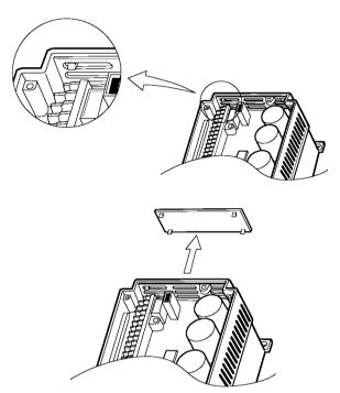
Figure 2-2-4 Removing the ventilating cover
