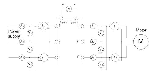
8-4 Insulation Test Avoid testing an inverter with a megger because an insulation test is completed at the factory. If a megger test must be completed, proceed as described below. Use of an incorrect testing method may result in product damage.
